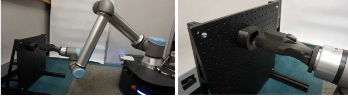
Figure 3.1: Experimental setup for plug insertion using a UR10e manipulator.
